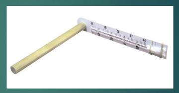
A <u>rain gauge</u> is used to collect <u>precipitation</u>.
