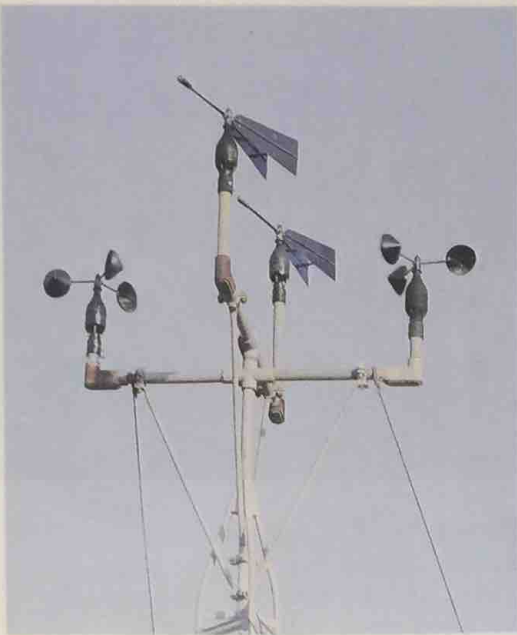
Figure 1-20 Wind speed is related to the rate at which the cups of the anemometer revolve. What other weather instrument can you see in the photograph?
